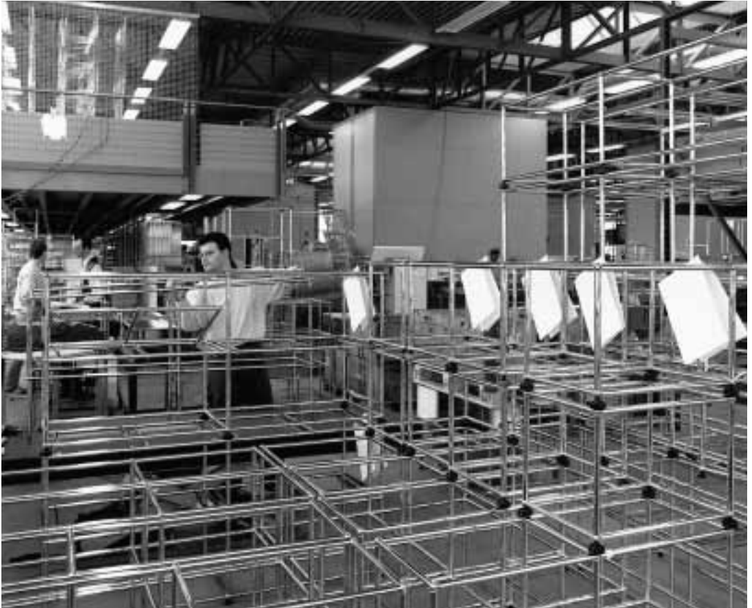
Pre-assembly of the frames
